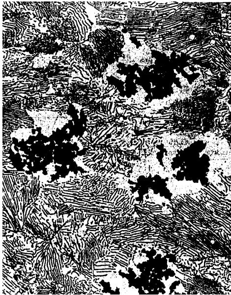
Fig. 1 Microstructure of a typical malleable cast iron showing graphite in the form of temper carbon. 4% picral etch. 250×
